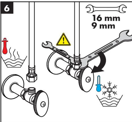
Connect the hot and cold supply hoses to the stops.
