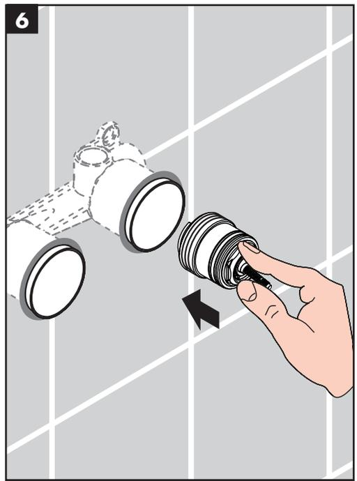
Install the cartridge assembly.
