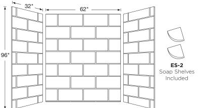
Designed to fit base areas 32" deep or smaller x 62" wide x 96" high or smaller (813 mm x 1575 mm x 2438 mm)
