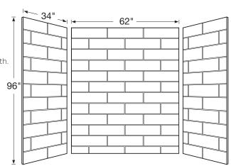
Designed to fit base areas 34" deep or smaller x 62" wide x 96" high or smaller (864 mm x 1575 mm x 2438 mm)
