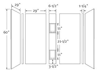
Designed to fit tub area 30" deep x 60" wide (762 mm x 1524 mm), or smaller
