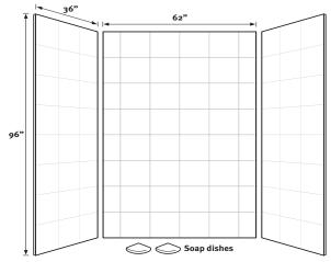
Designed to fit base areas 36" deep or smaller x 62" wide x 96" high or smaller (914 mm x 1575 mm x 2438 mm)
