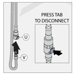
4) Attach outlet end of pull-down hose (V) to hose adapter (U).
