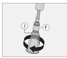
7) Remove spray wand (J) from pull-down hose coupling (F).
