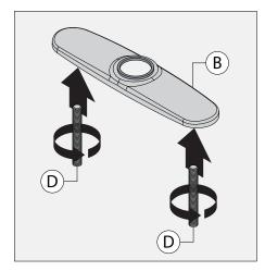
1) Thread studs (D) into deck plate (B).
