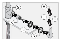
Replace cartridge (K), compression nut (L), collar (N), handle (O), set screw (I) and plug button (H).
