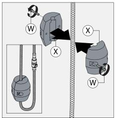
5) Attach counterweight (X) to outlet end of pull-down hose. Counterweight should be placed above the hose loop. Secure with 2x screws (W).
