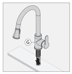
2) Install faucet body (G), supply hoses and pull-down hose to deck surface.
