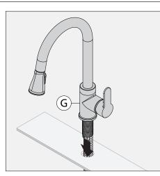
2) Install faucet body (G), supply hoses and pull-down hose to deck surface.
