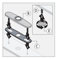
Install deck plate (B) and gasket (C) to deck surface. Thread mounting nuts (E) to studs (D) to secure deck plate (B) under deck.
