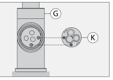
Inspect cartridge (K) for debris and replace cartridge if necessary. Align pegs on cartridge (K) with holes in faucet body (G) as shown above.
