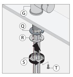
Install rubber washer (Q), metal washer (R) and mounting nut (S) to faucet body (G). Secure to bottom of deck with 3x mounting screws (T).
