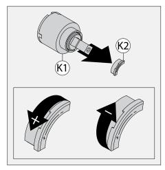
2) Remove limit stop (K2) from cartridge (K1). Turn limit stop counterclockwise to allow full handle turn to the hot position. Turn limit stop clockwise to limit handle turn to the hot position.
