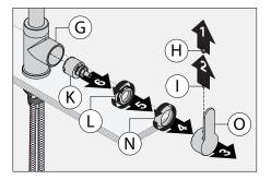
Remove plug button (H), set screw (I), handle (O), collar (N), compression nut (L) and cartridge (K) from faucet body (G).
