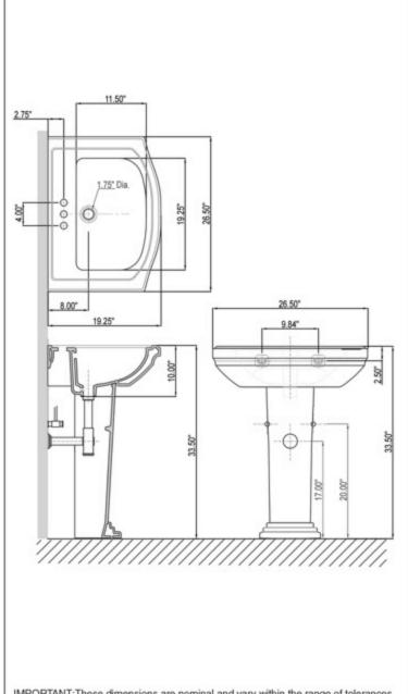
IMPORTANT: These dimensions are nominal and vary within the range of tolerances established by ASME standard A112.19.2
